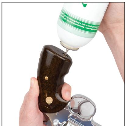
Place the gun base upward. Align the gasbottle with the valve and press down to fill the gun with gas.
