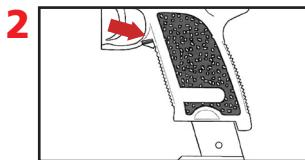
Push the magazine release button and pull out the magazine.
