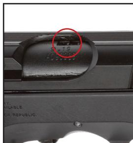
Gradually turn the adjustment dial towards "Hop" and fire a round or two to see the effect. Continue to adjust until the BBs fly straight/ horizontally. Perfect Hop-up is applied when the BBs fly straight.
