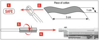
Put the safety on "safe". Prepare a thin rod with a length of approx. 30 cm. Attach a piece of cotton fabric to its end and clean the barrel with some silicone oil.
